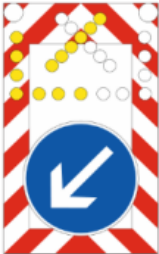
Figure 6-4 Mobile Signage for Blocking Lanes (RSA, 2021)
